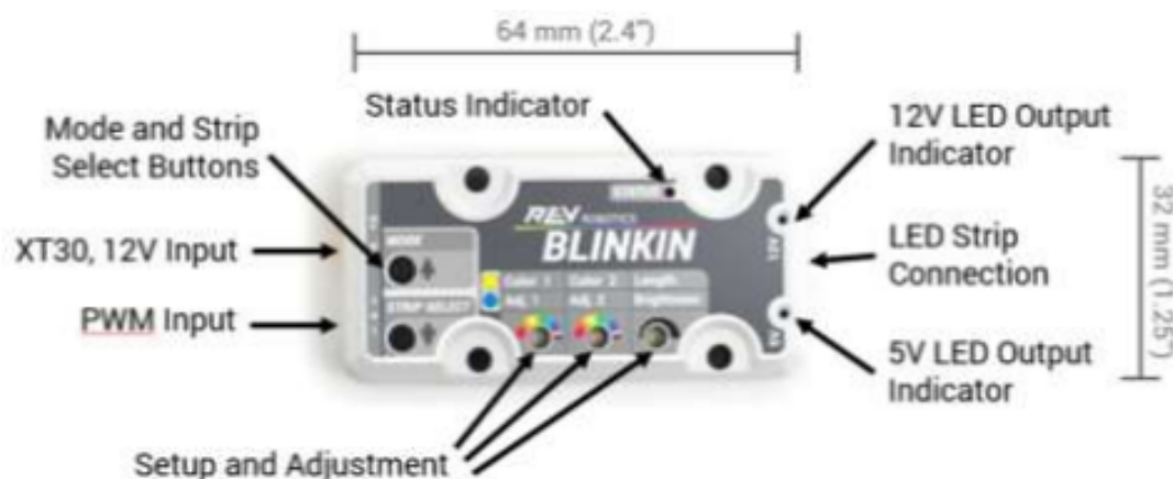
Figure 1: Blinkin Connections and Indicators
