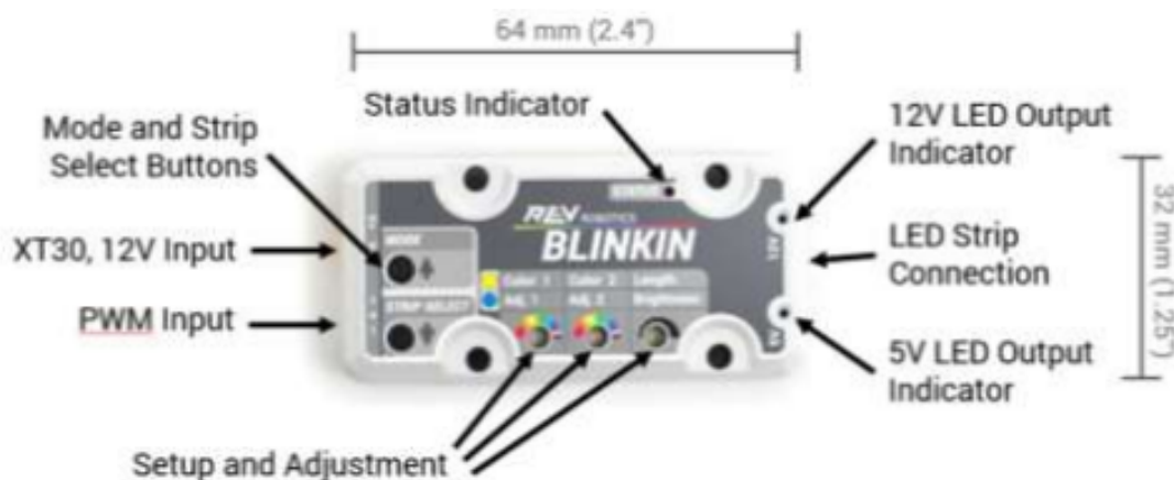
Figure 1: Blinkin Connections and Indicators
